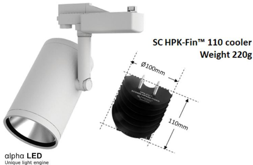
Figure 7: alpha LED™ Metropole from Projection Lighting Ltd using FrigoDynamics® SC HPK-Fin™ 110 2-Phase heat exchangers and Xicato 2000lm XSM LED modules. alphaLED™ is a registered Trademark of Projection Lighting Ltd
